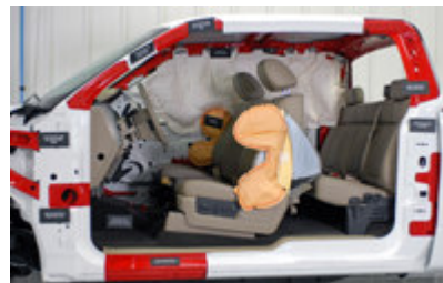
The all-new 2009 Ford F-150 – which features patented “K-bag” side air bag technology.
